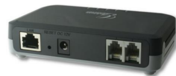
Fig. 2. Interfaces of ATA HT702 for connection from one side to the LAN, and on the other side, to analog terminal devices.
