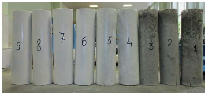
Figure 1. Specimens of PTC structures in a plastic tube: 1–3 — unencased specimens; 4–6 — specimens in a polyethylene encasement; 7–9 — specimens in a polypropylene encasement.
