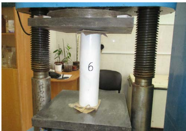
Figure 2. Specimen of a short TC bar before testing.
